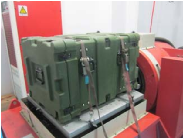
Vibration Test Photo
